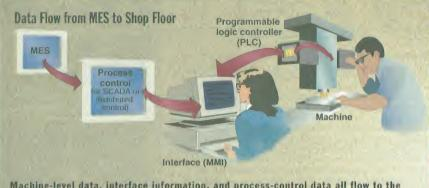
Machine-level data, interface information, and process-control data all flow to the MES for processing and distribution to other information systems.
